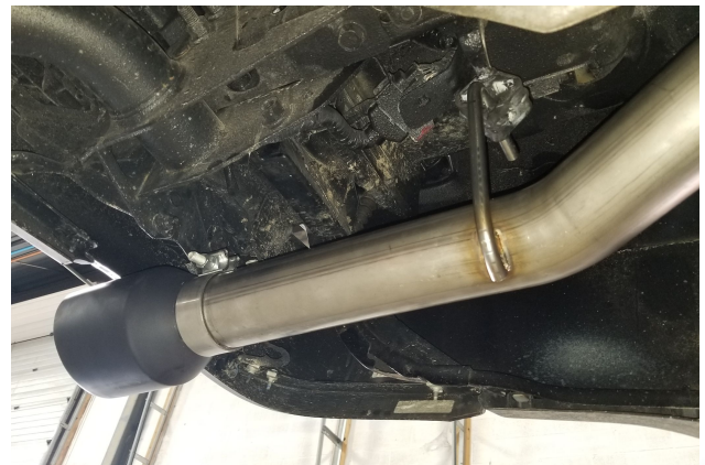
Detail 12: Rear tail section and tip installed.
