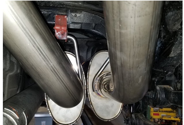
Detail 12: Orientation of hanger assemblies behind mufflers.
